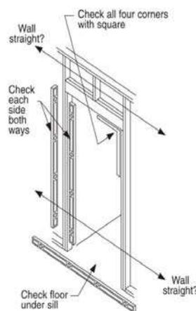
Is the opening the correct size for the door unit? Check it against the door frame size now, before installation. The opening should be frame height plus 1/2 inch, and frame width plus 1/2 inch to 3/4 inch. **Fix any problems now.**
