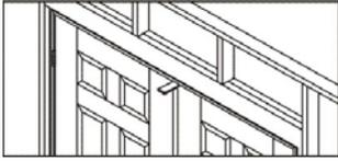
Place *temporary* shims above the center of the head frame, where doors meet. Pre-drill and insert a screw through frame into header, then remove the temporary shims.
