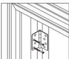
With the door open, drill 1/8 inch diameter pilot holes in the top hinge in the 2 screw hole locations closest to the weatherstrip. Then, install the #10 X 2-1/2 inch screws (provided) through the hinge, into the stud, to anchor the door frame and prevent sagging.
