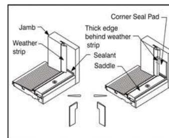
Apply sealant (Polyurethane or Elastomeric) at the joint where the threshold cap meets the door jambs.
