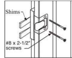
Then open the door and drill 1/8 inch dia. pilot holes and install the #8 X 2-1/2 inch screws (provided) through the strike plate holes to secure the lock side jamb and provide security.
