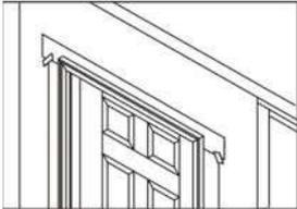
Provide and maintain a properly installed cap or head flashing to protect top of surfaces from **Water intrusion** and damage. Tape and properly seal the top flap of the Water Resistive Barrier (WRB) over the head flashing.
