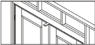
Shim above the mull post(s). Pre-drill and insert a screw through the frame into the header, at either side of the post.
