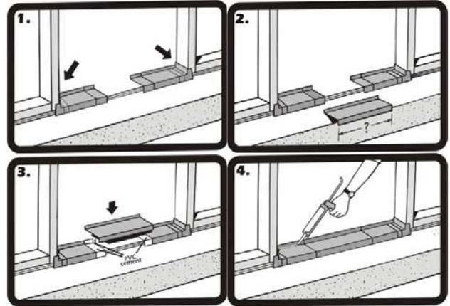
**Note:** Use only the PVC cement provided in the sill pan kit to glue the pieces together. The sill pan must be sealed to the sub-floor using an Elastomeric or Polyurethane sealant, but do not apply sealant to the bottom of the sill when using a sill pan.
