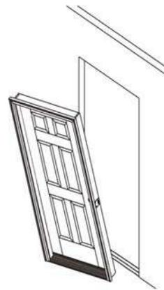
Lift the unit up. With top edge tilted away from opening, center the unit and place sill down onto sill pan or caulk beads and tilt into opening.
