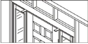
Shim above mull post or jambs separating doors and sidelites. Screw through the frame into the header, adjacent to the shims.
