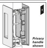
c) Repeat the process with the other side handle, taking care to line up the alignment pins with the two holes in the side handles and the third hole in the snib button (only applies to privacy handles) (diagram f).
