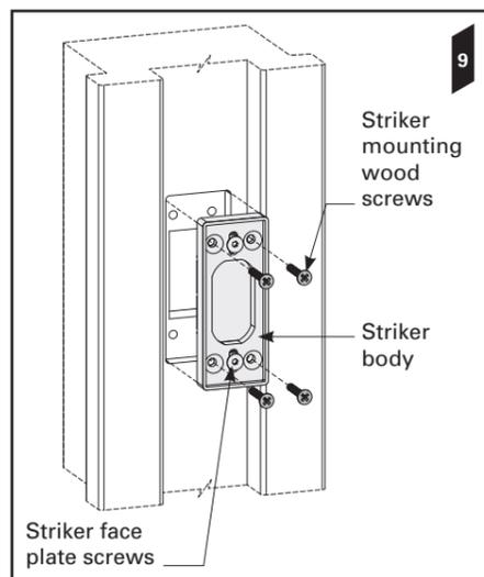
**10.** Remove the *striker face plate screws*. The *striker nuts* are now trapped in position.
