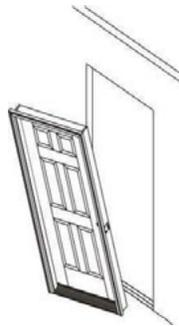
Lift the unit up. With top edge tilted away from opening, center the unit and place sill down onto sill pan or caulk beads and tilt into opening.
